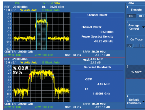
Simultaneous measurement of POWER and OBW
