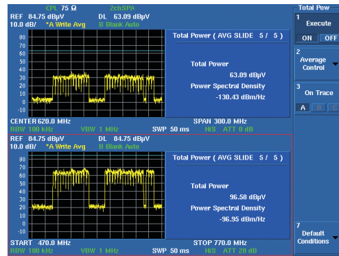
Simultaneous measurement of input/output for feed-forward amp
